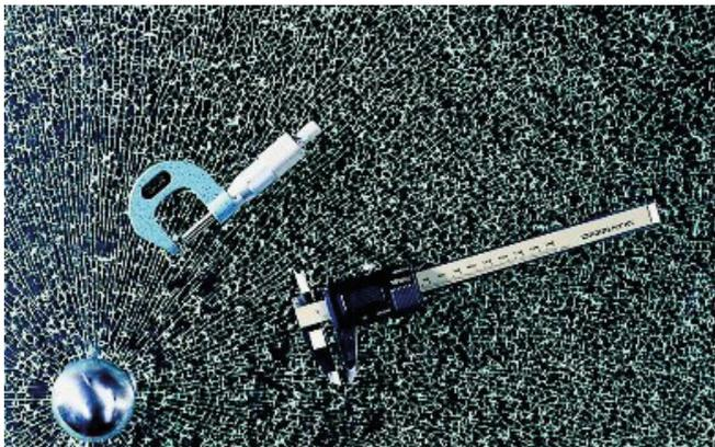
Safety glass (ESG) is produced in a thermal process. After being mechanically processed the glass is heated up to more than 600° C with a rapid cooling afterwards. Compressive stress on the glass surface and tensile stress within the glass ensure an increased impact strength and shock resistance. In case of breakage there are just small crumbs which reduces danger of injury.
